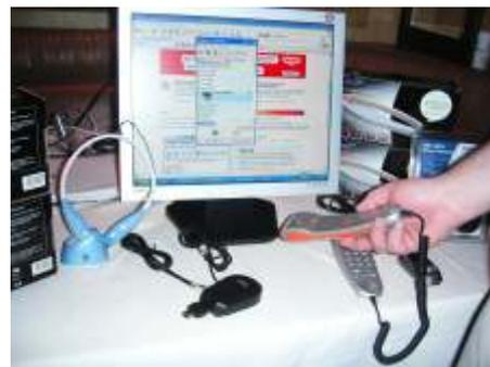
functions used with Skype are accessed direct from the unit itself. The keypad enable users to scroll through their list of contacts, adjust the call volume, and mute calls. Simply lifting the handset from its base automatically opens the Skype application on the computer screen. Acoustically isolated speaker and microphone eliminate echo. Available online for \$60.
