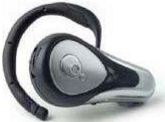
**Flamingo** it's weight is 8 grams, there is a standby time up to 130 hours, and 8 hours of talk time. It uses Bluetooth for connectivity.
